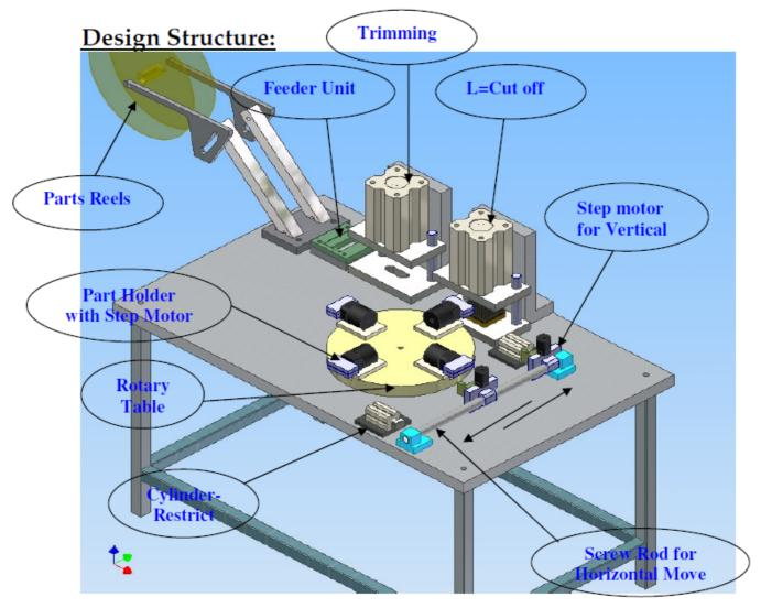
Process flow for Auto Pin Insertion Machine
